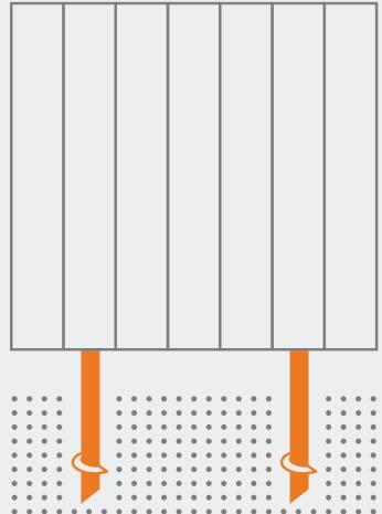
Whether you are considering a light garden fence or a heavy noise reduction barrier, screw piles can be a great choice. With the right conditions and machinery, and a competent team, screw piles can be installed in a matter of minutes. The use of adjustable brackets can make the job even easier. Installing the screw pile's helix to a frost-free depth easily negates the need for frost protection.
